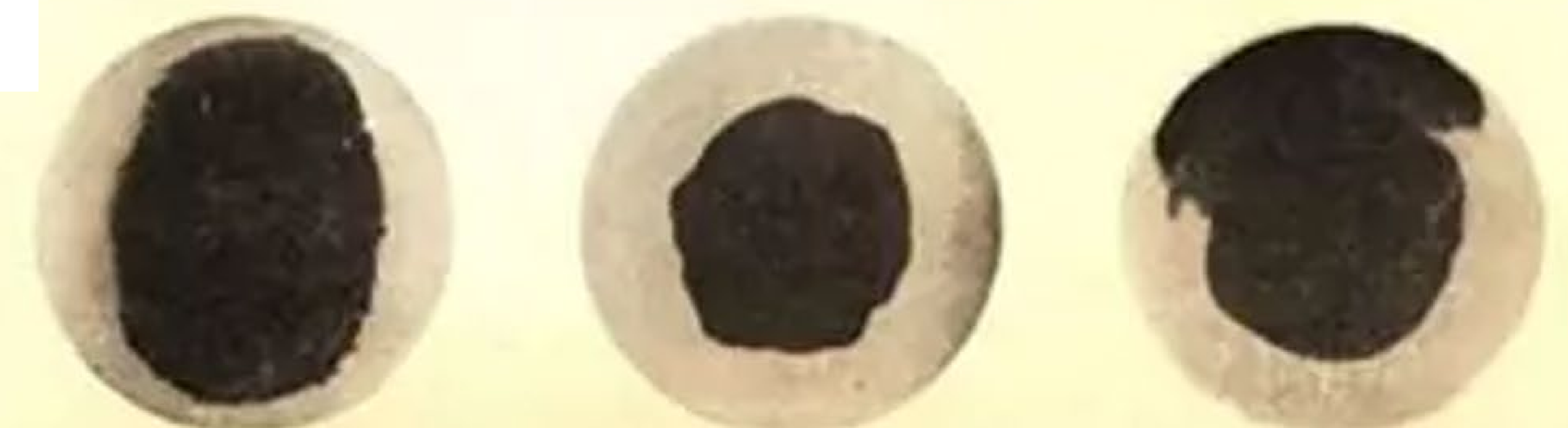
Unretouched X-Ray photographs showing balls with distorted centers
